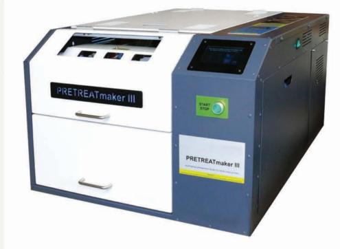
The Blizzard Pre-treat Maker III for direct to garment digital printing has an advanced electronic system to give an extreme performance and easier control during operation. The colour touchscreen allows easy setup of the spray length, width and the easy control of pre-treatment volume used. The machine is equipped with four valves (nozzles) which can each be controlled individually.
